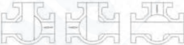
Several service conditions for which the ordinary “T” pattern floating three-way ball valve is not suitable
